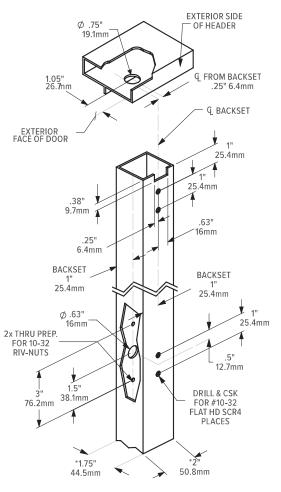
\* Preparation and installation of 4576 devices are based on 1.75" x 2" stile external dimensions. Doors with a thickness other than 1.75" will require modification to the 4576 device.
