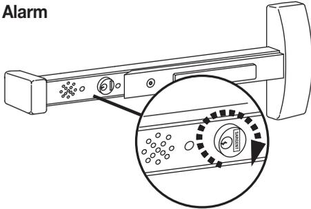
Turning key clockwise, the yellow PASSAGE LED will flash for 15 seconds (default), then a quick chirp and the ARMED green LED will flash and repeat every 30 seconds. Signal above cylinder indicates unit is armed.
