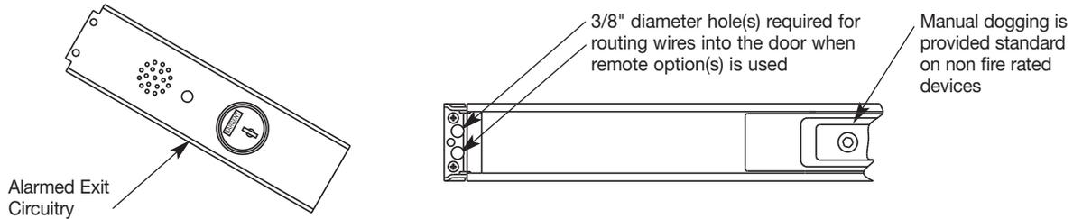
\*Field cut rail assemblies are not allowed. Exit Device must be ordered from the factory for specific door width.
