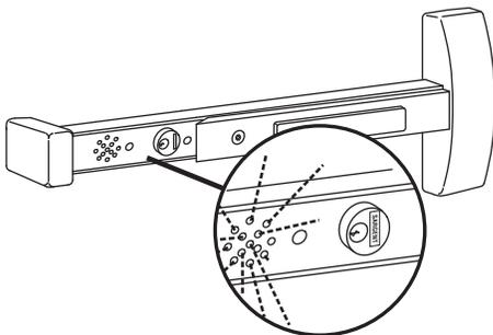
Horn chirps intermittently to indicate low battery condition. Change battery.
