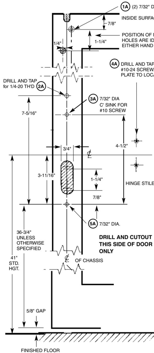
Door prep shown is the same for all less bottom rod 8400 Exit Devices, except the 12-NB-MD-8400 requires the thermal pin supplied.
