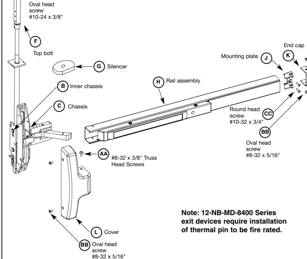
**Note: 12-NB-MD-8400 Series exit devices require installation of thermal pin to be fire rated.**
