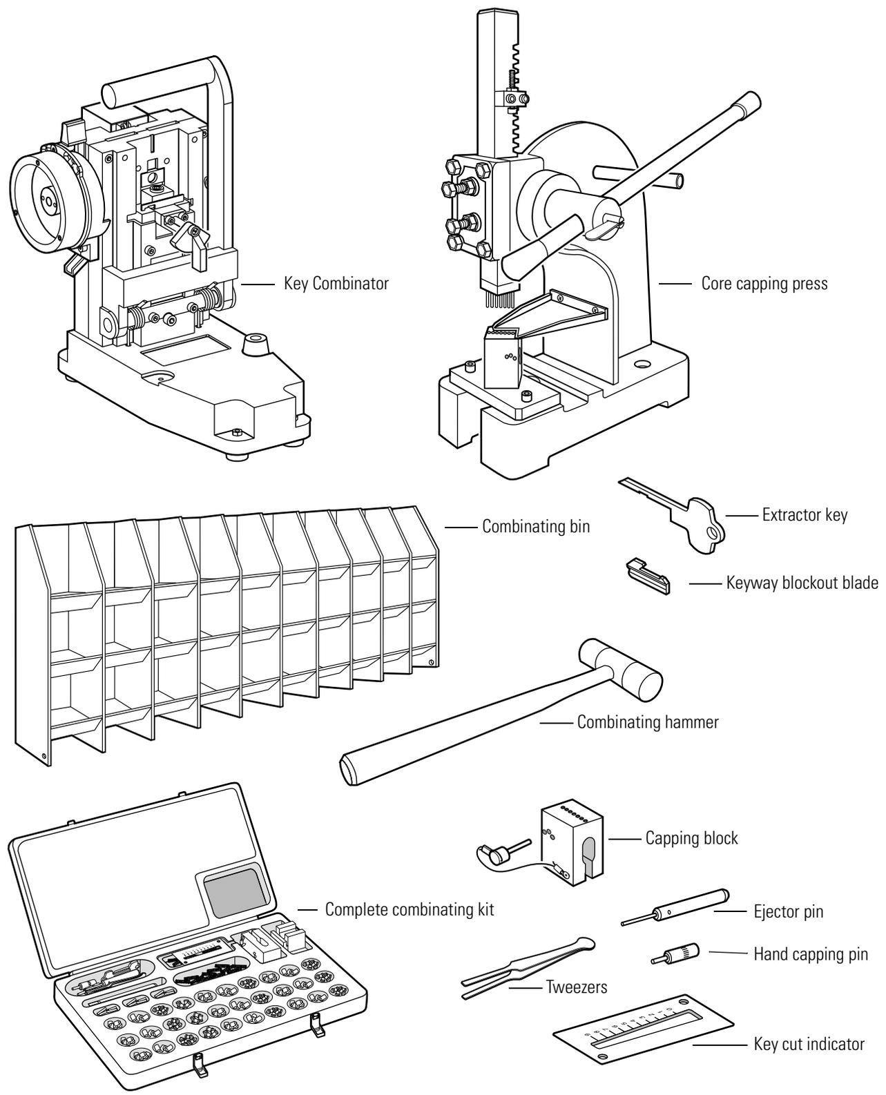
**Figure 3.4** Tools used for servicing cores and keys
