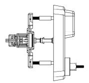
Note: Lever not shown must be installed prior to installing trim to door and chassis.
