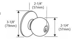
Knob projections shown are for 1-3/4" (44mm) thick doors and will vary by door thickness.
