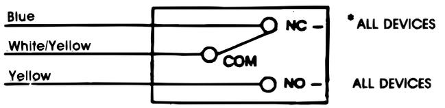
**"O" MONITOR** – Device actuated SPDT switch to indicate door open from outside.
