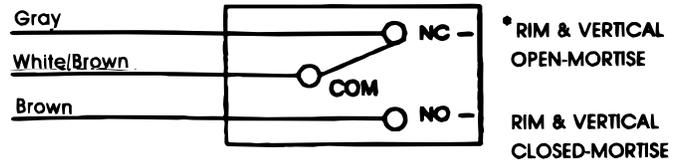
**"S" MONITOR** – Slider actuated SPDT switch to indicate bolt(s) extended-retracted.
