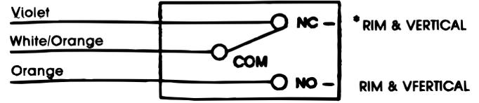
\* SWITCH POSITION WITH DOOR SECURE AND DEVICE LATCH ENGAGED.
