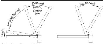
**Closing Speed Valve** (1/8 Allen Wrench Provided) To adjust speed of door closing from fully open to a position 2" to 5" from closed, turn Closing Speed Valve CLOCKWISE to SLOW closing, COUNTER-CLOCKWISE to SPEED closing.
