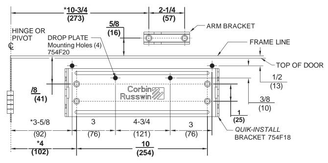
To obtain extra closing force add 3 (77) to dimensions marked. This will limit degree of door opening to 130°.
