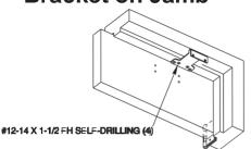
Using holes spotted on soffit or stop in Step A mount adapter plate bracket.
