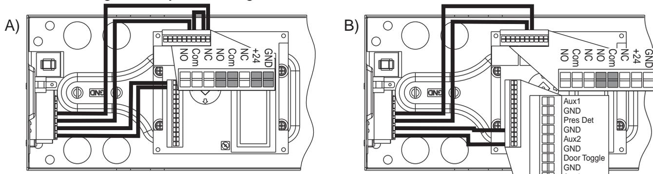
**Electric Latch Retraction Exit Device Wiring - Blow Open**
