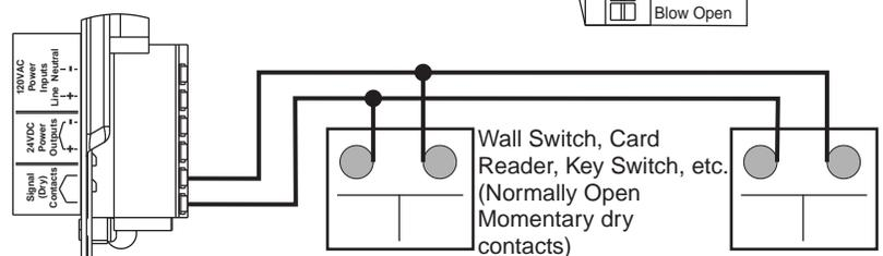
**Electric Latch Retraction Exit Device Wiring**
