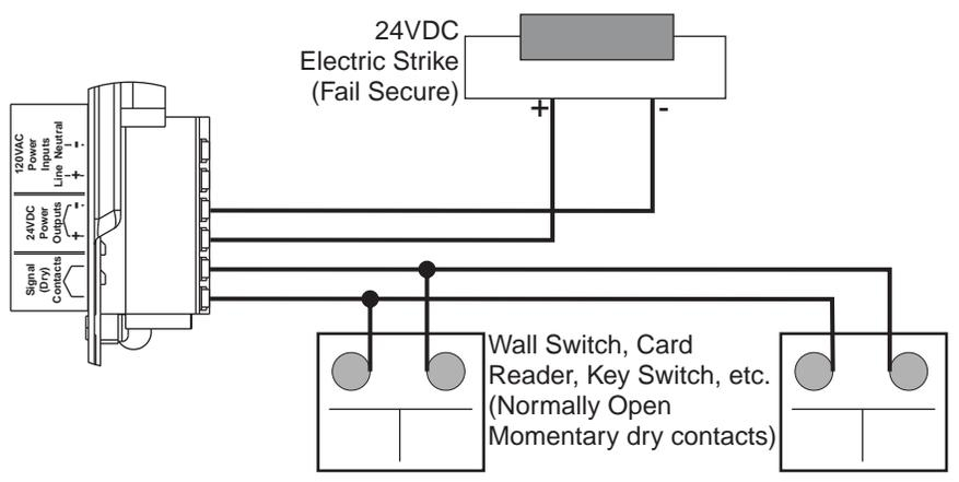
**Electric Latch Retraction Exit Device Wiring**
