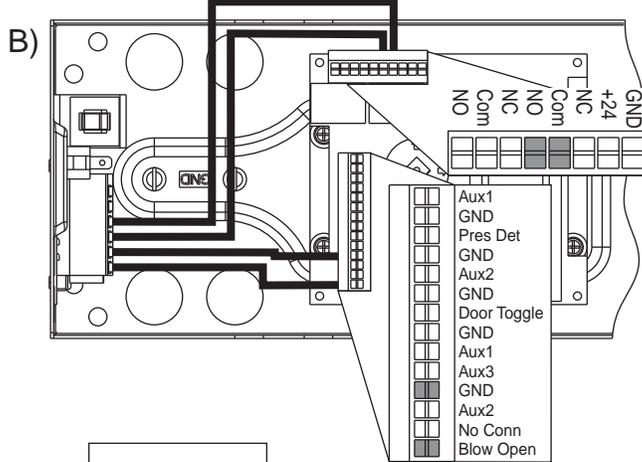
**Electric Latch Retraction Exit Device Wiring - Blow Open**
