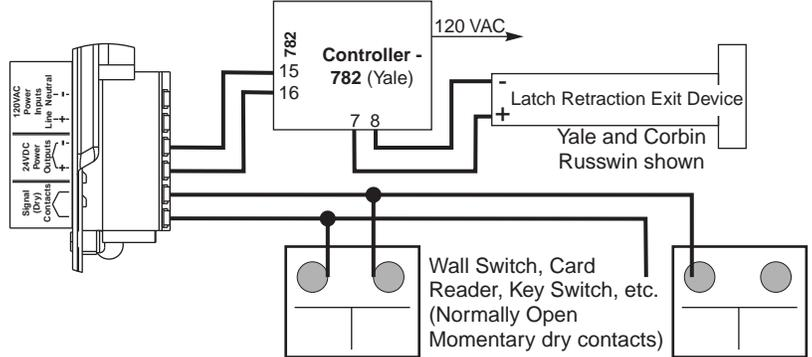
**Electric Latch Retraction Exit Device Wiring for Smoke Ventilation - Blow Open Function**
