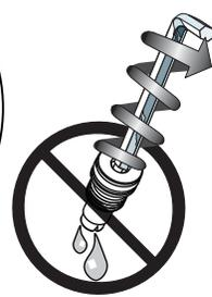
Do not remove valves from closer. Hydraulic oil will escape.
