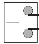
Wall Switch, Card Reader, Key Switch, etc. (Normally Open Momentary dry contacts)
