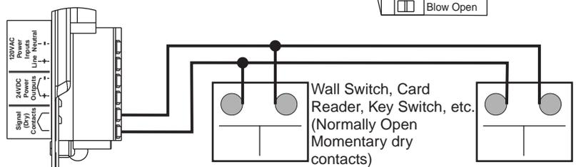
**Radio Frequency Standard Function Wiring (can be ordered pre-wired to this RF wiring)**
