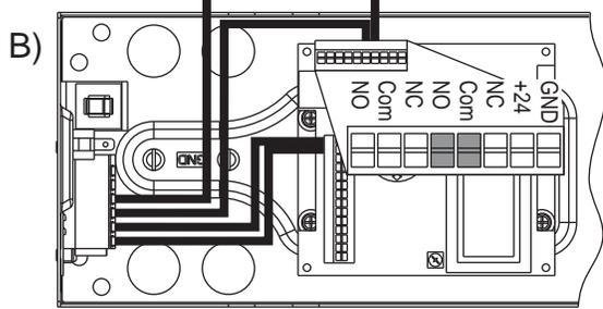
**Electric Latch Retraction Exit Device Wiring**
