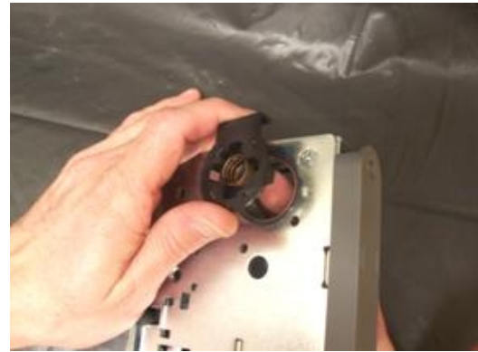
Step 1. Remove Cylinder Monitor Assembly from Lockbody by gently pushing up through the opposite side of cylinder hole.
