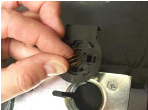
Step 2. Remove spring from assembly. Use caution not to stretch or otherwise deform the spring.
