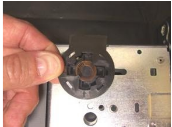
Step 8. Install spring into assembly. Use caution not to stretch or otherwise deform the spring.
