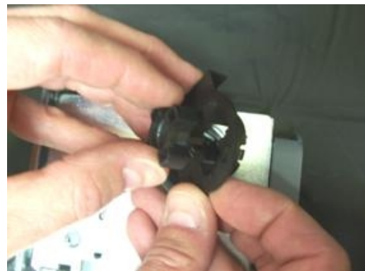
Step 3. Remove Inner Shell from Outer Shell by gently pressing the Inner Shell upwards from the bottom. Use caution not to damage sensor wires.
