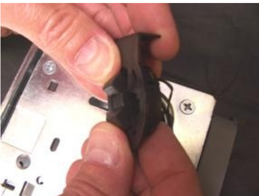
Step 4. Turn Inner Shell on side. Align the inner shell with the diagonal slot in the Outer Shell. Slide the Inner Shell through the Outer Shell.
