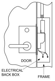
Electric Actuator. Solenoid points up when actuator is used
