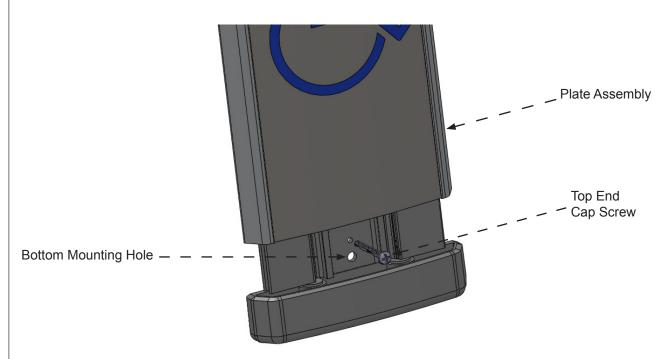
With the bottom mounting hole now exposed, plumb the plate assembly and install the bottom mounting screw. Remove top end cap screw from base while supporting the front plate. Slide the front plate back down. Replace top end cap with the provided screws and insert push-in plastic screw caps.
