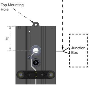
Plate assembly and end cap removed to show cable routing.
