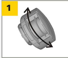
Adjust the **lateral position** of the detection field.
