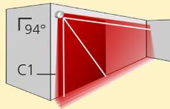
The distance between the inner curtains of the 2 sensors must be max. 8 in to ensure safety according to EN ISO 13849-1:2008 CAT 2, Pl «d».
