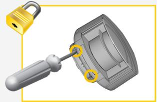
**Lock the position** of the mounting bracket to avoid malfunctioning in case of extreme vibrations.
