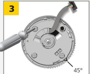
Position the bracket and fasten the 4 screws firmly in order to avoid vibrations.
