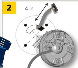
Pass the cable +/- 4 in through the cable opening. If drilling an opening is not possible, use the cable conduits on the back side of the bracket.
