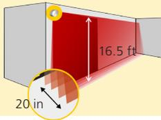
The visible laser beams indicate approximately the position of curtain C1.
