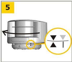
Position the housing on the bracket and turn the sensor until the two triangles are face to face.
