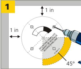
Use the mounting template to position the sensor correctly. The grey area indicates the detection range. Drill 4 holes and make a hole for the cable if possible.
