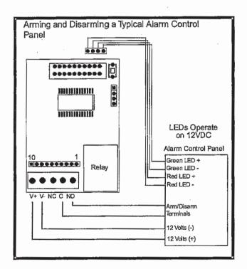
To control the LED's externally cut the four wires going to the green and red LEDs. Each LED'has a black and red wire. Black is the negative and red is the positive. These LED's require 12VDC to operate.
