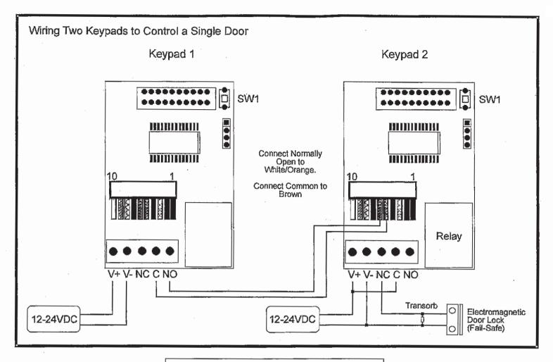
The diagram above shows how to connect two keypads to control a single door. Entering your code on keypad 2 unlocks the maglock directly. When you enter your code on keypad 1, it triggers the REX input of keypad two, which unlocks the door.
