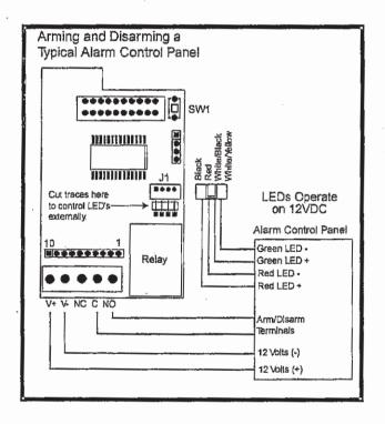
To control the LED's externally cut the four traces in the box underneath connector J1. Before connecting the alarm panel's LED control lines to J1 verify the traces are cut. To verify, measure continuity between the end of the wire on the wire harness and the square pad on the circuit board below the box corresponding to the wire you're measuring. Permanent damage to the keypad may result if voltage is connected to J1 when the traces are not cut.
