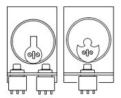
Select shape of cam shown for no. of switches used (specify when ordering cylinder).
