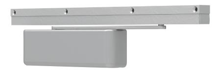
The 4510T Smoothee Series is a heavy duty, high security track closer with special components to minimize tampering and vandalism. Forged steel single lever arm and heavy gauge metal security cover are designed for correctional, vandal prone, institutional and other high traffic interior applications. A choice of finishes and cylinder functions meet correctional and vandal resistant requirements.
