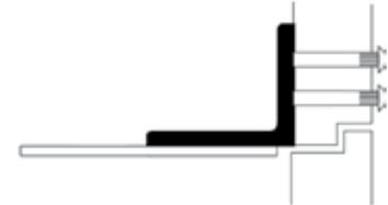
**Standard - #2019S Spacer Block:** For use where a narrow frame soffit does not provide adequate support for the soffit plate. Supplied as standard with all CloserPlus® arm closers. For use on frame with either 1/2" (13mm) or 5/8" (16mm) high frame stop.
