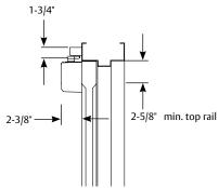
The pull side application of the 422 cam closer provides an aesthetically pleasing appearance with the functionality of pull side mounting. In the pull side application, the closer body mounts to the face of the door and the track mounts to the face of the frame. All cam action closers are equipped with a short track which provides superior door control with a clean appearance.
