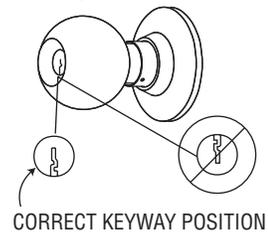
A. Verify keyway is in the downward position. If not, proceed to steps 9B through 9D.
