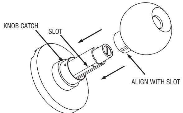
B. To install inside knob, align inside knob with slot and push all the way down until knob locks in place.
