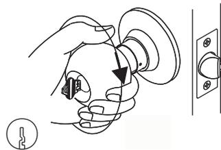
B. Insert key in cylinder. Turn knob clockwise until the Knob Catch appears in the small hole. Use key to ensure cylinder remains in the vertical position.
