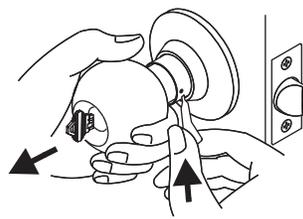
C. Using catch release tool, press the knob catch and pull the knob off.
