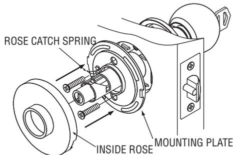
A. Rotate mounting plate so rose catch spring is facing opposite the lock stile and slide on until flush with door. Tighten machine screws securely to install mounting plate. Press rose onto mounting plate. Be sure to fit rose in recess of mounting plate.
