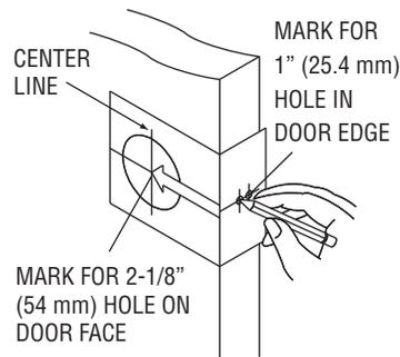
Measure center line of lock; height as desired from finished floor. Select 2-3/4" or optional 2-3/8" backset, fold and apply template to high side of bevel of door and mark center of door edge as indicated on template. Mark center hole on door face through guide on template.
