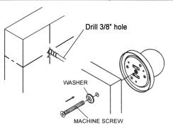
Measure centerline of lock height as desired from finished floor. Measure backset as desired from door edge and mark centerline. Drill 3/8" hole through door. Insert machine screw through door and tighten securely with knob.
