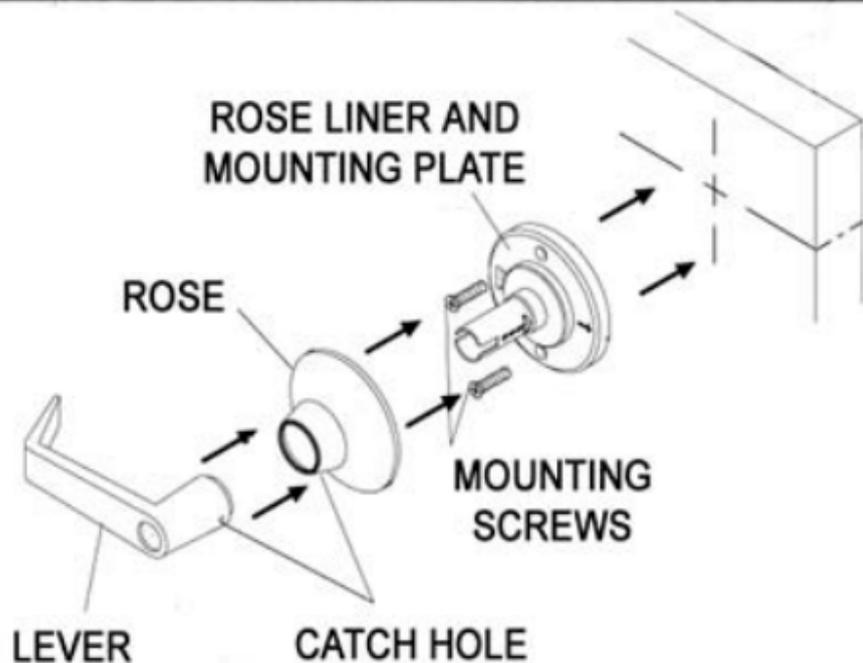
Measure centerline of lock height as desired from finished floor. Measure backset as desired from door edge and mark centerline. Together, press mounting plate and rose liner against door and tighten screws. For metal doors, drill and tap for #8-32 size screw. Press on rose and handle.
