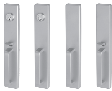
512TP 512NL 512DT 512TP-BE 717DT Escutcheon: 16" x 2 3/4" Grip: 6 1/4" C-C Projection: 2 11/16" Brass For keyed functions, see page 14 for cylinder requirements.
