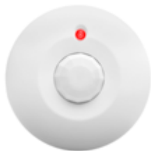
PYR-3011 Wireless Ceiling PIR Motion Detector • Digital electrical and magnetic protection: distinguishes between electrical interference and real temperature changes • Detection range: 7-m (23-ft) diameter, 360° @ 2.4-m (7.9-ft) height
