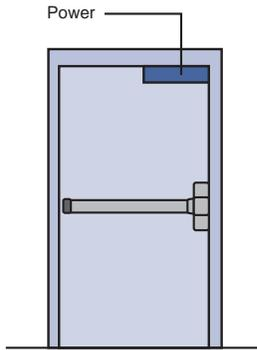
Door Movement Trigger by Latching Exit Device
