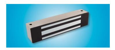
Magnetic lock providing 600lbs of holding force: fully sealed electronics are protected from water and dust, surface mounted with minimal tools, mounted using steel machine screws into finishing nuts, ten feet [3.05m] of jacketed, stranded conductor, operates with 12 or 24V DC power
