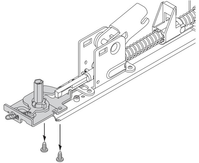
2. Drill or use center punch on two rivet heads until rivets can be removed from baseplate.
