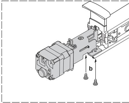
**7** Install Mechanism Case
