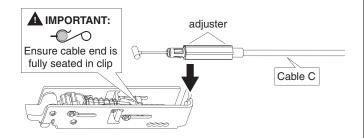
Temporarily Attach Bottom Latch Cable Assembly to Center Slide.
