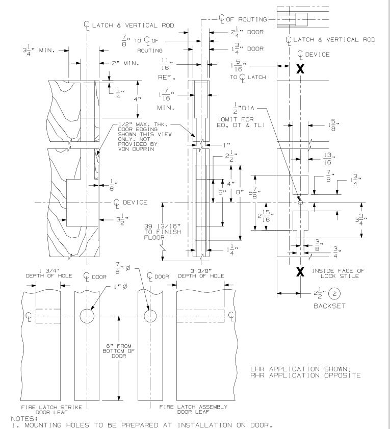
1. MOUNTING HOLES TO BE PREPARED AT INSTALLATION ON DOOR.
