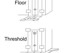
For threshold application, remove roll pin and fitting, cut bottom rod, reinstall fitting and roll pin in second hole
