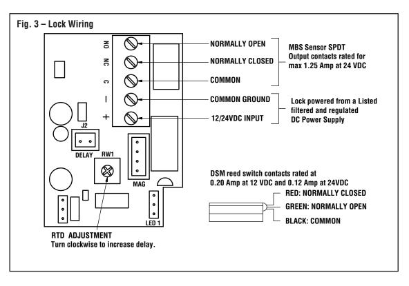
6. To Ensure Instant Release All switching devices must be wired in between the DC power source and the positive terminal of the lock in Fig. 4. Switching the negative power supply line will not allow the lock to release immediately.
