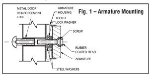
**NOTE:** During the installation of the armature plate to the door it is essential that the armature plate remains movable. The armature plate must be allowed to pivot on the center-mounting bolt to allow proper alignment with the magnet surface. If the plate is not aligned with the magnet surface, the lock may lose holding force or not lock at all.
