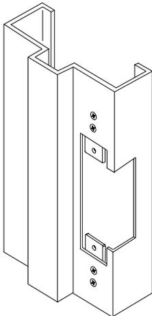
**4** Shim strike in or out as needed until faceplate is flush with frame.
