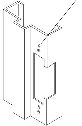
**3** Mount the two mounting tabs inside frame using #10-24 screws as shown below.
