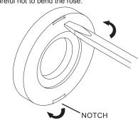
Note: Inside Rose has a notch to aid removal when installed. Please position this notch towards the bottom of the lock assembly.
