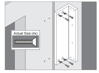
2b Attach mounting bracket to L-Bracket.
