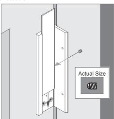
3c Attach armature holder to second TJ bracket.
