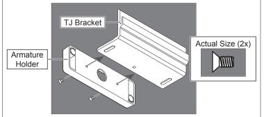
3d Attach armature plate to armature holder.
