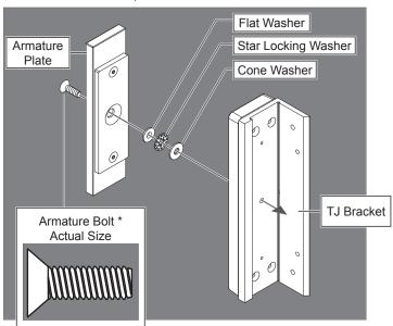
\* Armature bolt must be tightened to 120 in-lbs. Replace with bolt in Gate kit. M490 armature must be disassembled to replace armature bolt.
