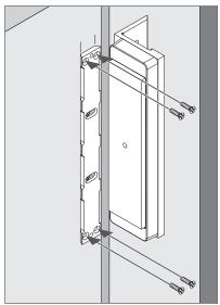
3f Reinstall magnet and secure with two screws.
