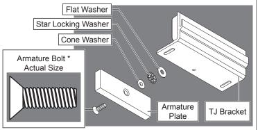
\* Armature bolt must be tightened to 120 in-lbs. Replace with bolt in Gate kit. M490 armature must be disassembled to replace armature bolt.
