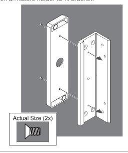
2b Attach armature plate to armature holder.
