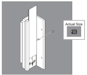
2d Attach Armature Assembly to moving part of gate.
