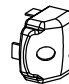
EC2 Endcap (AL) (for FCA): P/N 104686-X EC2 Endcap (S.S.) (for FCA): P/N 104317-X
