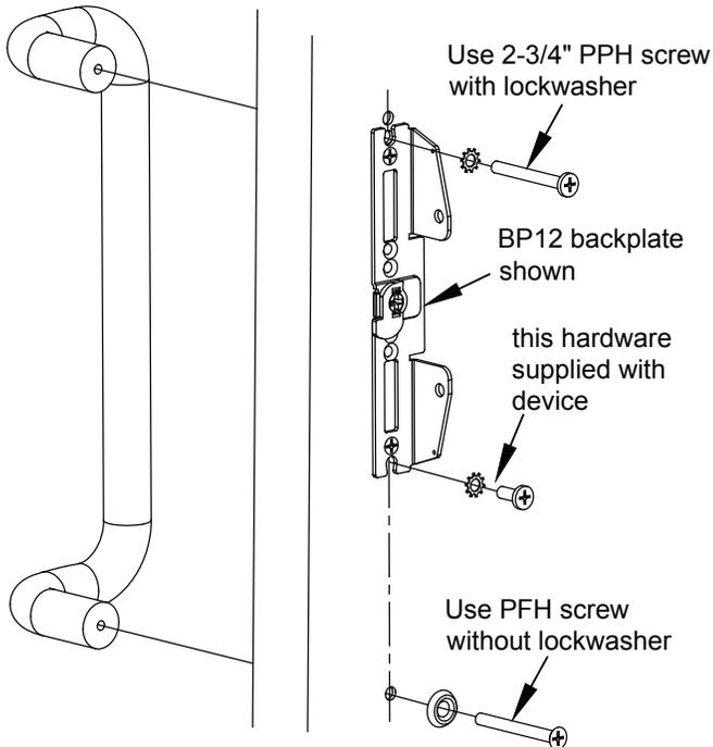
Wire Pull mounted beside\* device vertical  $\varnothing$ .
