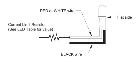
NOTE: Use heat shrink to protect resistor connections from shorting
