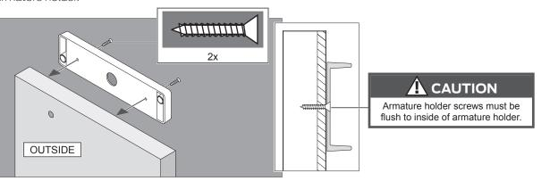
2b Install armature plate as shown for door type (M420/M450 shown).
