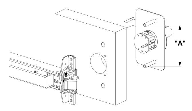
3)IF"A" ABOVE IS 3-1/2", PREPARE THE HOLES MARKED **"B" (INSTEAD OF "A")** IN THE INSTALLATION INSTRUCTIONS. IF "A" ABOVE IS 4-1/2", PREPARE THE HOLES PER THE INSTALLATION INSTRUCTIONS.
