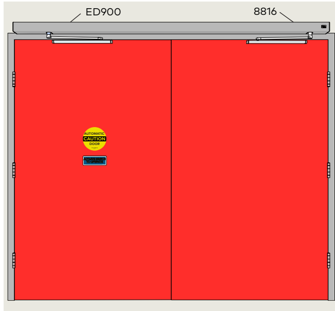
Fig. 32.2.1 Companion door installation
