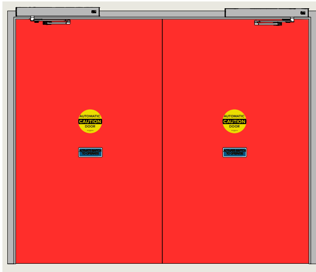
Fig. 32.2.1 ED900 low energy installation
