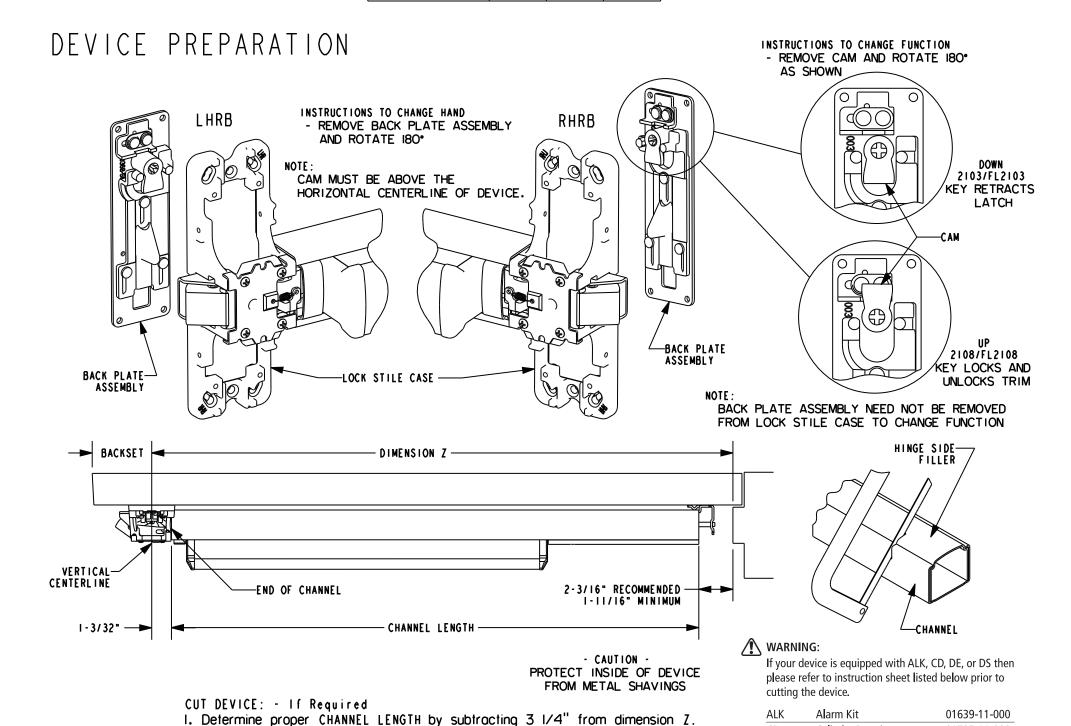
2. Mark cut off point (hinge side filler must be all the way inside of channel).
